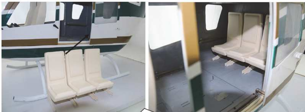
Glue back seats 【62】 into place as shown.
