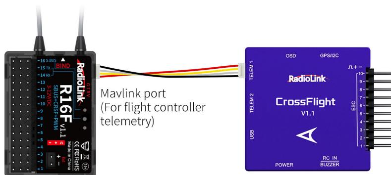
Mavlink port of R16F is connected to the TELEM port of RadioLink CrossFlight
