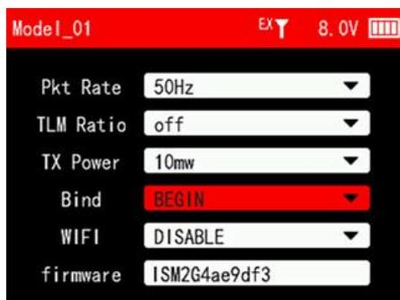
7. After the binding is successful, the signal tower will appear in the upper right corner, and the LED of the ELRS receiver is always on.
