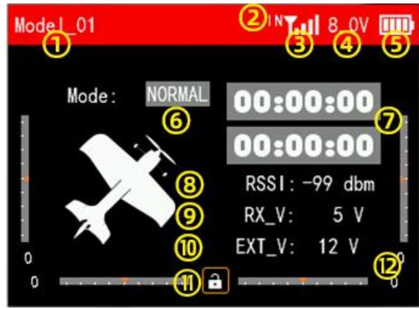
Long pressing the power button of T12D to turn it on, the screen will display as shown below:
