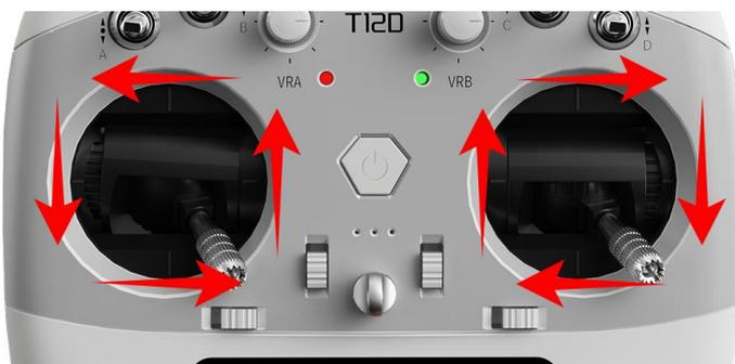
Turn the knob, VRA and VRB, clockwise to the maximum, and then counterclockwise to the minimum. Refer to the picture below:
