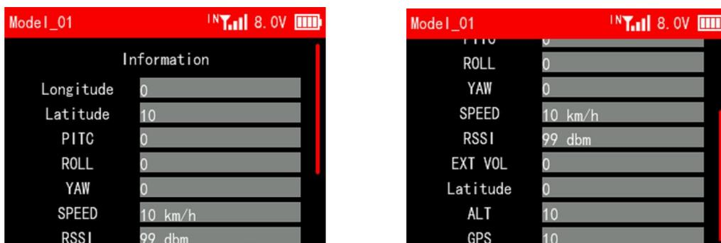
When T12D works with a R16F receiver, a flight controller and a GPS, connect the Mavlink port of R16F to the TELEM port of the flight control (See picture below) and set the relevant parameters in Mission Planner to get the flight controller telemetry on the screen of T12D.
