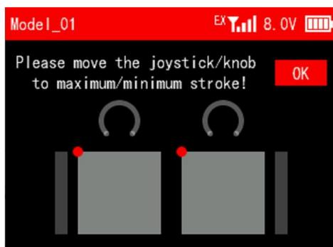
Push the two joysticks to the lower left corner, lower right corner, upper right corner, upper left corner respectively. Refer to the picture below:
