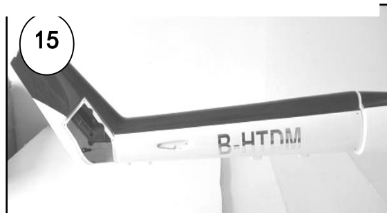
When installed the Transition Tail Gear Box, whirligig the tail for 90°.
