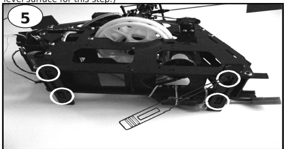
5 Place the Plastic Spacers onto the landing gear position of the heli mechanism and secure it using M3x14mm Hex Cap Screws with \phi 3x \phi 8x0.8mm spacers.
