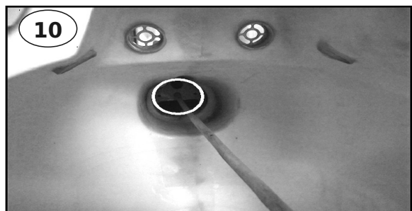
10 When inserting the Heli Mechainsm into the Scale Body, make sure the Scorpion Tail Shaft pass through the front 10mm hole inside the Main Tail Part of the scale body.
