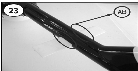
Glue the Horizontal Stabilizers onto the Main Tail Part using epoxy. (Remarks: Keep two Horizontal Stabilizers in equal Horizontal level.)
