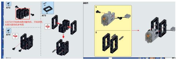
Install the servo in step A72 as shown below.
