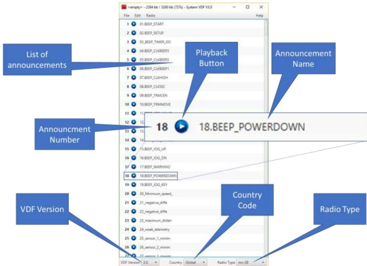
On the bottom of the window, there are combo boxes to select the VDF version, the country code and the radio model.
