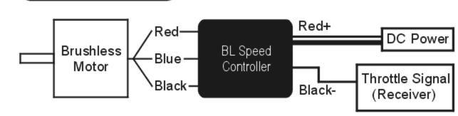
Exchange two wire for changing motor rotation direction.
